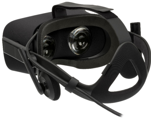
Figure 1: Oculus Rift, first consumer version (CV1). Image source: Wikipedia 4
